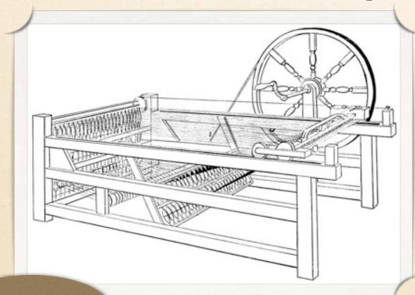
This machine is called a Spinning Jenny. It enabled yarn to be produced much more quickly than with a single spinning wheel. They were used in textile mills.
